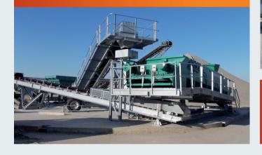
LOG WASHERS with a tub length up to 8,000 mm
