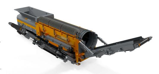
Featuring a self-cleaning screening drum, the TS175 Trommel Screen prevents buildup of material such as wet clay or soil and keeps your mesh clear for passage. The unique lift bar system in the drum allows material to be lifted and cut more easily as it passes through the trommel. With two hydraulic-powered conveyors, users can easily separate and stockpile materials.
